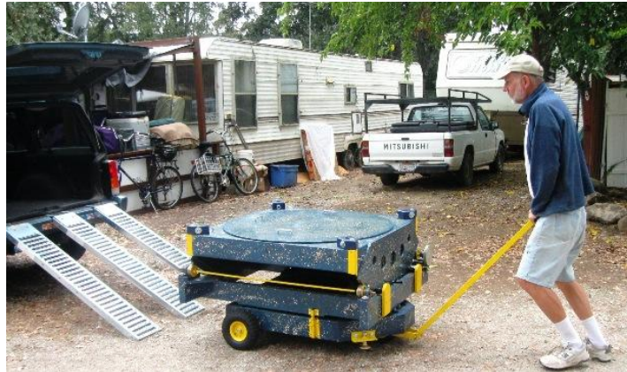
Russ and his wife Cheryl, a philosophy professor, stand beside Russ’ 1-meter portable telescope. For transport, the telescope, with its top truss structure disassembled, fits into the back of a Jeep Cherokee.
