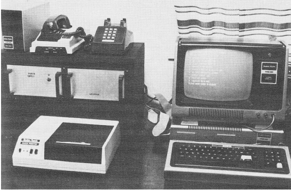
Figure 3. A Radio Shack TRS-80 microcomputer) was used for data reduction. Also shown are a thermal printer, modem, and (upper left) a floppy drive.
