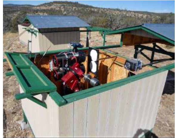
Figure 13. Tom Smith's Dark Ridge Observatory has two operational robotic telescopes. The twin astrograph is in the foreground and the 14-inch Meade is in the background (roof closed).
