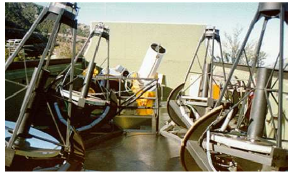
Figure 10. The three original robotic telescopes at the rear of the Fairborn Observatory are almost obscured by the four 0.8-meter telescopes that were subsequently added—completely filling up the available space. These seven robotic telescopes observed together harmoniously every clear night on Mt. Hopkins for many years.
