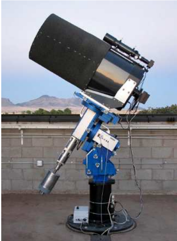
Figure 15. The 0.5-meter DEMONEX robotic telescope at the Winer Observatory observes exoplanet transits for Jason Eastman at Ohio State University.
