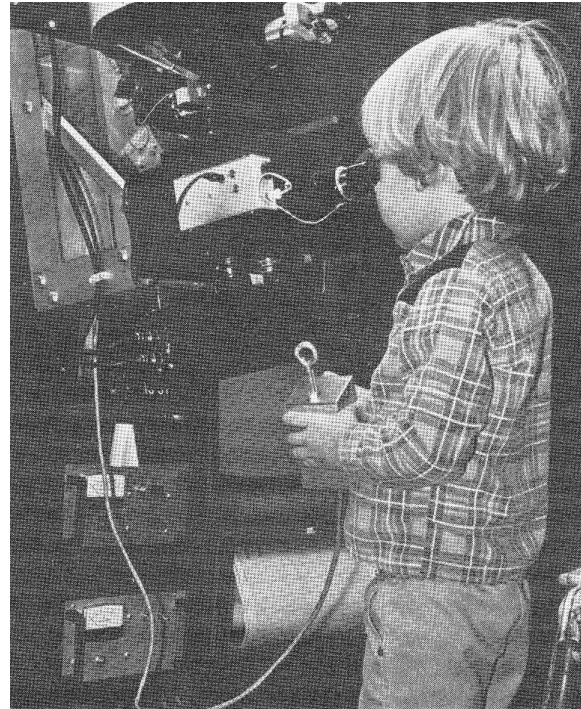
Figure 2. Russ Jr. (1979) centers a star at the Fairborn Observatory's first telescope. The UBV photometer, DC amplifier, high voltage power supply, and strip chart recorder are visible.
