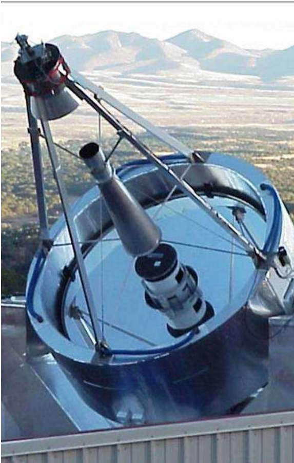
Figure 12. The 2-meter telescope at the Fairborn Observatory is dedicated to spectroscopic observations via a fiber-fed spectrograph.
