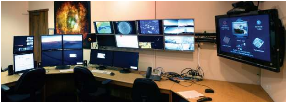
Figure 17. The remote controls for the Canada-France-Hawaii Telescope (also in Waimea) are now used to operate the telescope with no one actually at the telescope at night.
